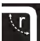
Min. bending radius ( $r$ ) = 15Ø
